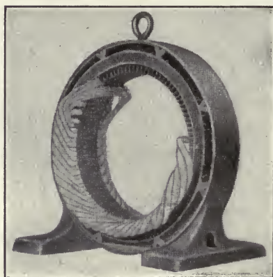
FIG. 142.—A three-phase stator partly wound with basket coils.
